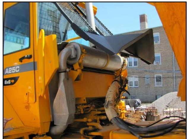
*Diesel Particulate Filters (DPFs) like the one pictured above when used with Ultra Low Sulfur Diesel (ULSD) can reduce emissions by 90%*
